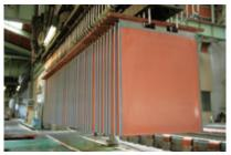
Refined copper produced using the permanent cathode method
