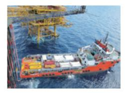
A supply vessel provides CO2 for injection into the reservoir
