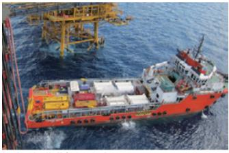
A supply vessel provides CO2 for injection into the reservoir
